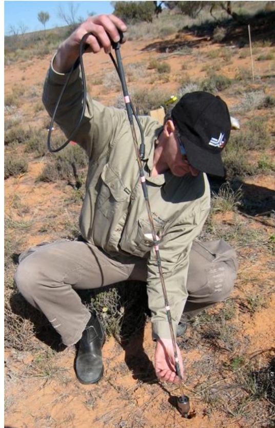
Figure 3: The author inserting thermistors into one of the probe casings fully inserted in the ground.
