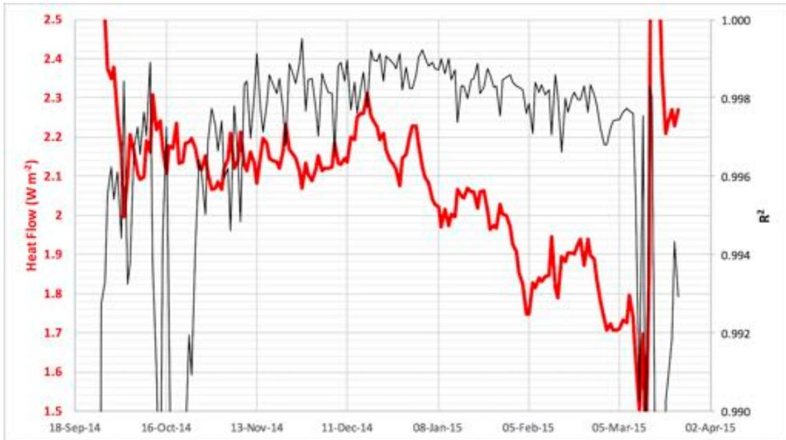
**Figure 29.** ‘Reduced surface heat flow’ versus time for site AZ2 (red, left axis); Coefficient of determination (black, right axis).
