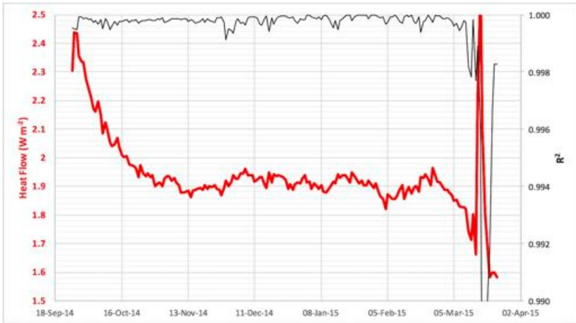
**Figure 40.** ‘Reduced surface heat flow’ versus time for site AZ4 (red, left axis); Coefficient of determination (black, right axis).
