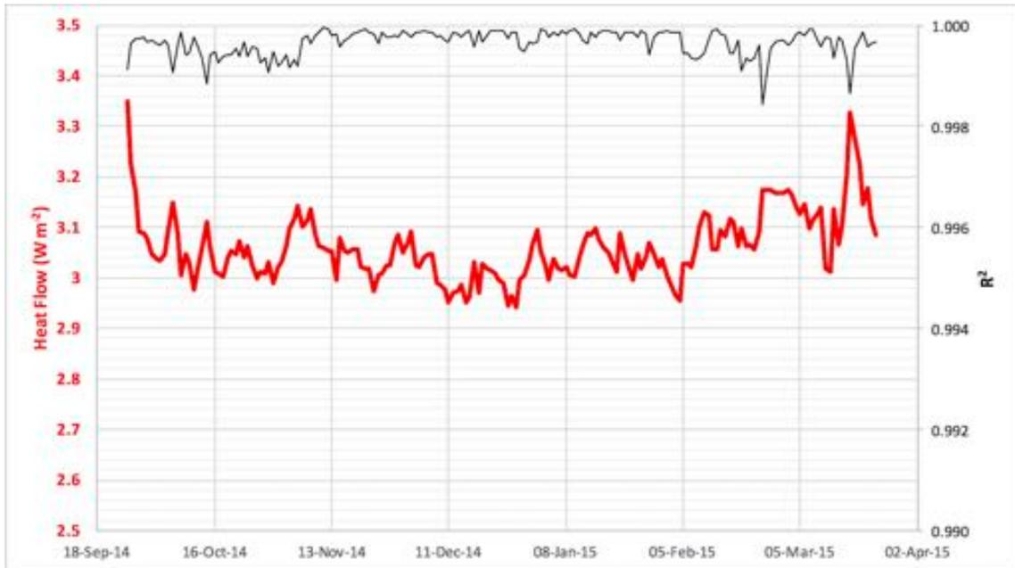
**Figure 51.** ‘Reduced surface heat flow’ versus time for site AZ6 (red, left axis); Coefficient of determination (black, right axis).
