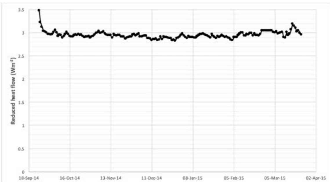
**Figure 6.** Reduced surface heat flow through time deduced from a Heat Needle record. The values in the first weeks of the survey are influenced by random errors in the surface temperature history, but equilibrate to a static  $2.9 \pm 0.1 \text{ Wm}^{-2}$ . No significant temporal changes in ‘reduced surface heat flow’ are seen in this case.
