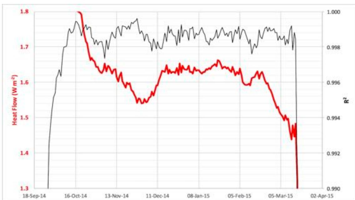
**Figure 18.** ‘Reduced surface heat flow’ versus time for site AZ1 (red, left axis); Coefficient of determination (black, right axis).
